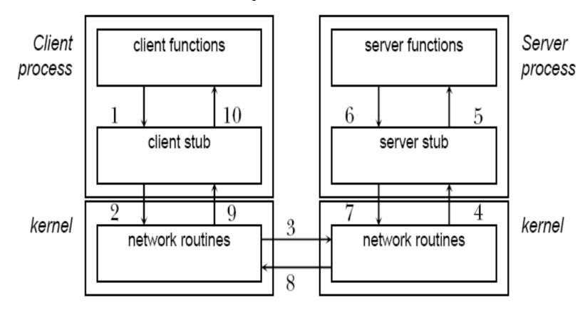
Step 5. The sever stub executes a local procedure call to the actual server function, by passing the arguments receivedStep 6. When the call completes, it returns values back to the server stub
