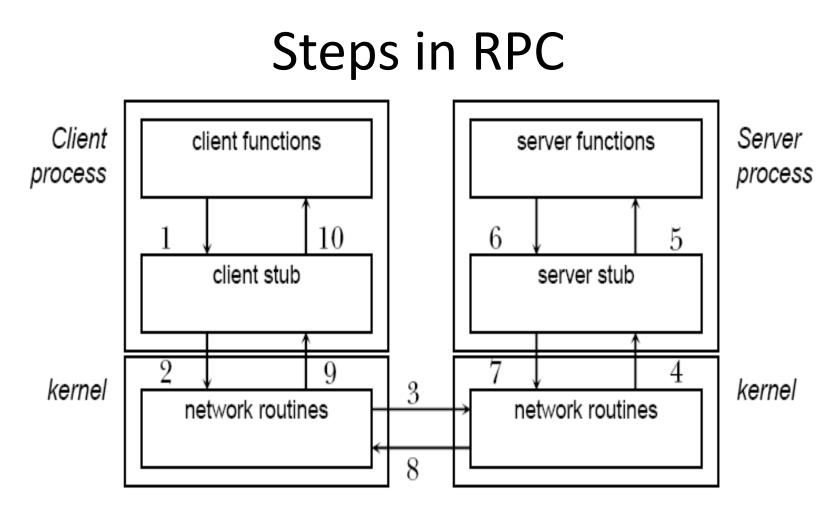
Step 7. The sever stub converts the return values (if necessary) and marshals them into one or more network messages to send to the client stub Step 8. Messages are sent to the client stub
