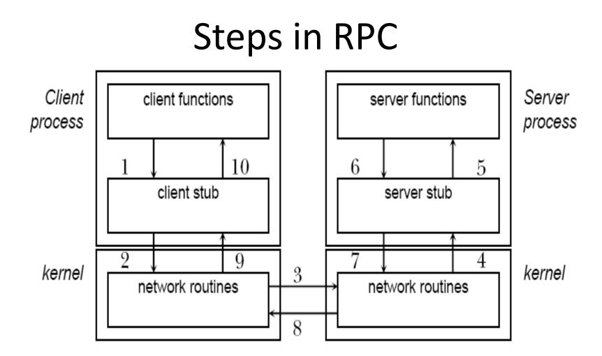
Step 1. The client calls the client stub which packaging the arguments into a network message (marshaling) Step 2. The network message is forwarded to the network routines (local kernel by system call)
